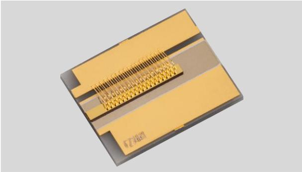
SkyEra delivers TY-975±10nm-45.0W-25C-COS-SIC-01 chip on submount diode lasers, employing AuSn bonding and P Down package with multiple advantages of high reliability, stable output power, high power, high efficiency, long lifetime and high compatibility, and are widely applied in the market.
