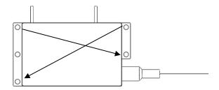
• First, apply thermal paste or other thermal materials evenly on the bottom of the product, thermal paste should not be too thick;
